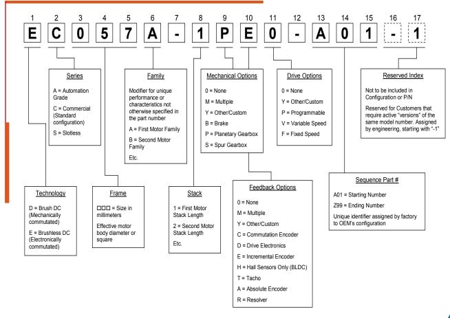
Finally, S indicates that the brushless motor is a slotless design.
