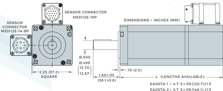
It's impossible to fully optimize dc applications with a limited range of off-the-shelf motors. AMETEK Pittman partners with the OEM's design engineers to tailor dc motors to specific applications. Shown here is one variation from dozens in the motor manufacturer's brushless dc motor series.
