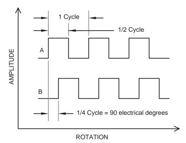
Figure 1: Two-channel incremental encoder waveform.
