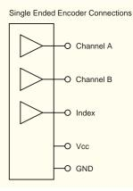
Figure 5: Connector pin-out for a three-channel encoder with single ended outputs.
